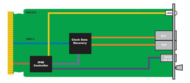
FIGURE 1. AMC214 Functional Block Diagram
